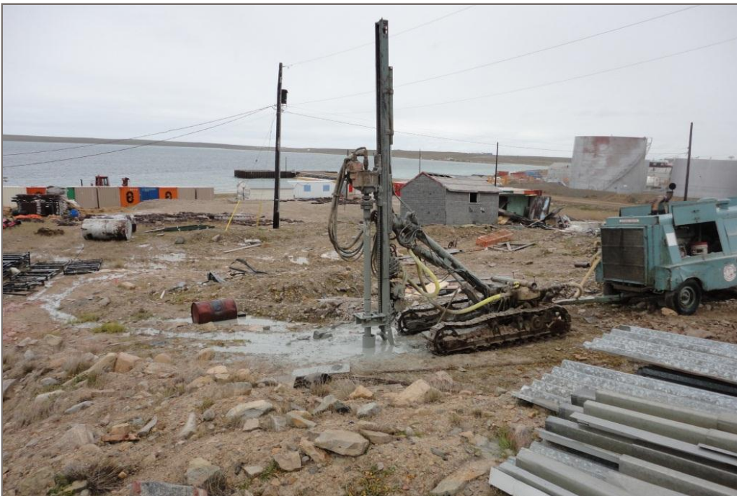
Photo 6: Air-rotary drill at Site C Probehole 07, looking southwest. Note water on surface discharged during drilling.
